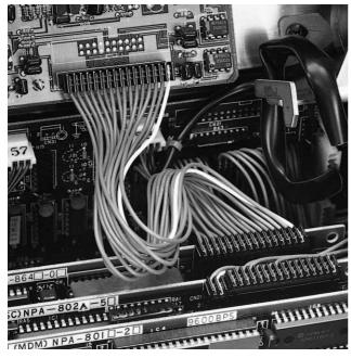
This 2.5mm (.098") pitch insulation displacement connector is another version of the NR connector for printed circuit boards. The NRD connector allows daisy chaining and is very useful in simplifying connection systems in electronic equipment.
